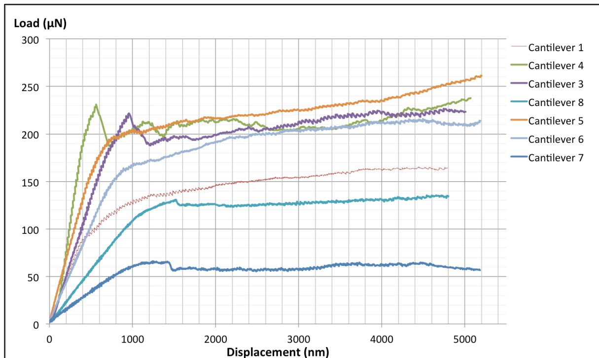
Figure 68: Load displacement curves for all cantilevers.
