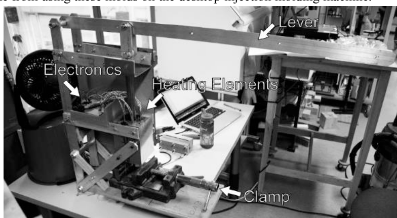
Fig. 2. The desktop injection molding machine in use: Clearly visible are the heating elements and the electronics, as well as the clamp for holding the molds. The long lever is for manually injecting the molten plastics.
