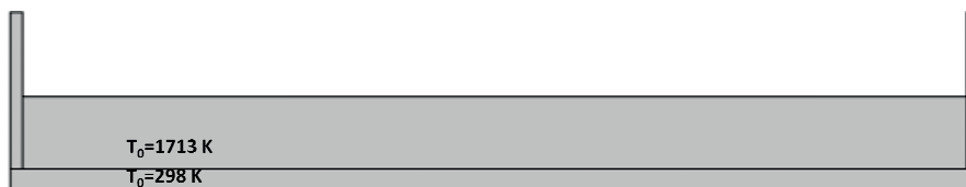
Figure 4.15: Sketch of the 2D geometry of the 30 mm cast from copper plate experiments. Mould dimension : 10 mm vertical and 400 mm horizontal. Silicon dimensions : 30 mm vertical and 390 mm horizontal. Graphite : 5 mm horizontal.
