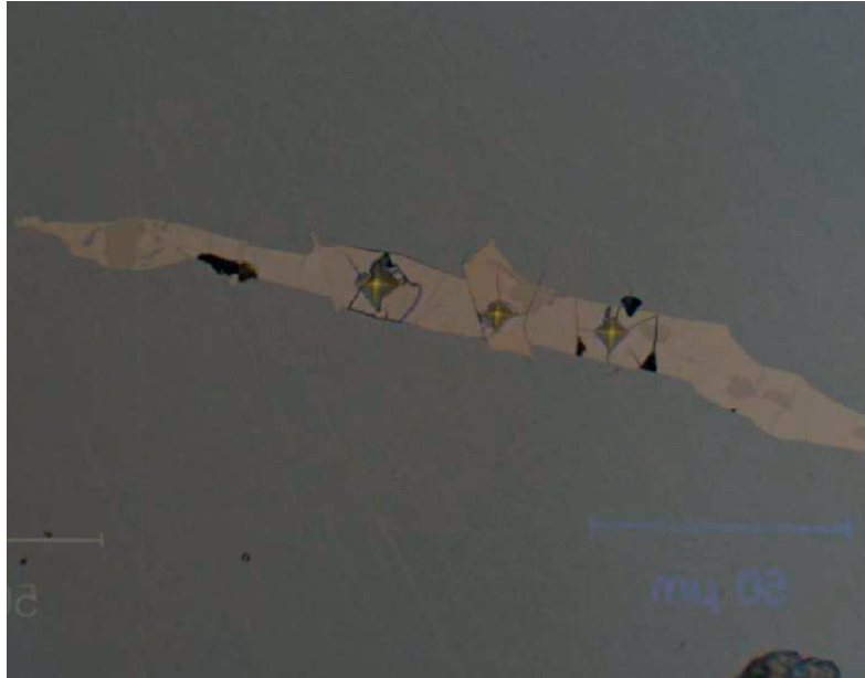
Figure 6.3: Light microscope image after micro hardness measurement.
