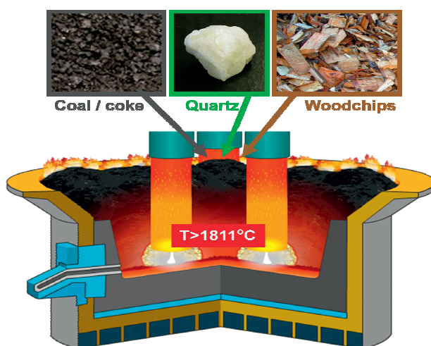
Figure 1.4: Illustration of the production of metallurgical grade silicon in an electric arc furnace from raw materials quartz, coal/coke and woodchips ( Elkem internal ).
