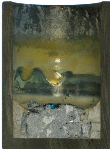
Figure 5.1: Cross-section of crucible after 6 hours experiment with the most silica-rich binary CaO-SiO<sub>2</sub> slag.
