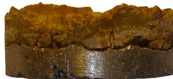
Figure 5.2: Cross section after complete removal of crucible from experiment with ferrosilicon containing 35% iron.
