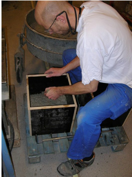
Photo 6-1 Casting of concrete cubes.
