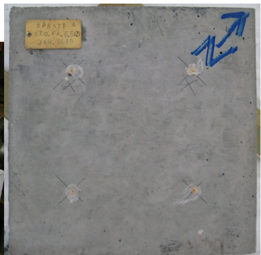
Photo 6-2—6-3 Preparation of measuring points (brass screws, glued in drilled holes; left) and final prepared cube including nameplate (right).
