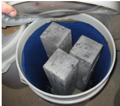
Photo 3-10 Storage containers for the Norwegian CPT (see details in paper IV, Table 3).
