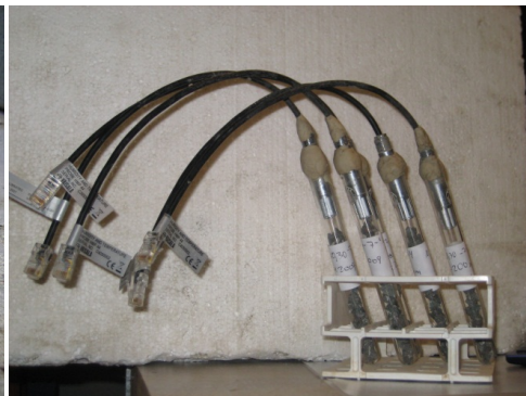
Photo 3-15—3-16 RF measurements; crushing of concrete (left) and glass tubes with Vaisala sensors (right).
