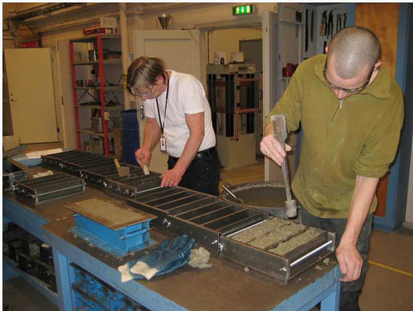
Photo 5-1 Casting of concrete prisms.
