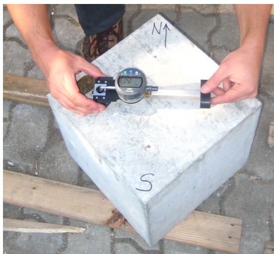
Figure 4. 200 mm digital Demec mechanical strain gauge.
