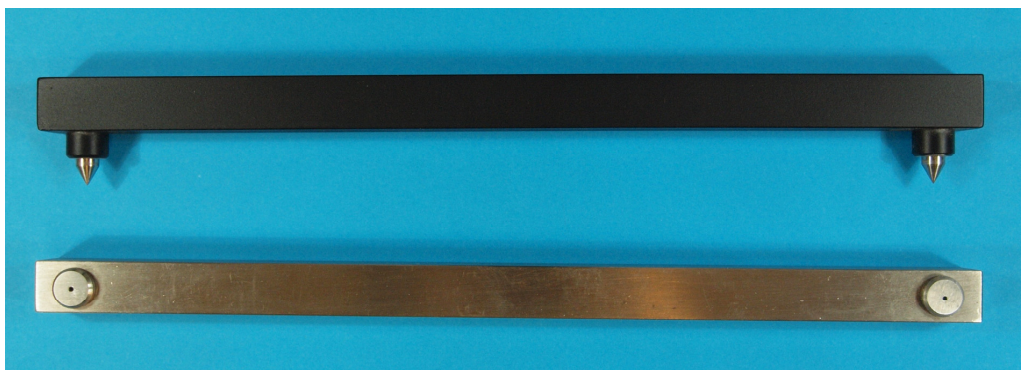
Figure 2. 200 mm “length marker bar” (black) and the 200 mm Invar reference bar.
