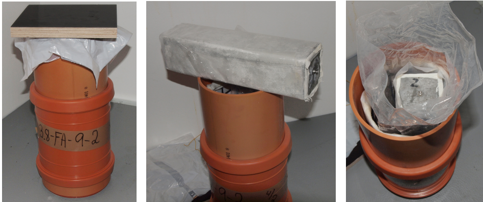
Photo 3-1—3-3 RILEM AAR-3: Storage container (left), wrapped prism (middle) and wrapped prism inside the prescribed polyethylene bag (right) (see details in paper IV, Table 3).
