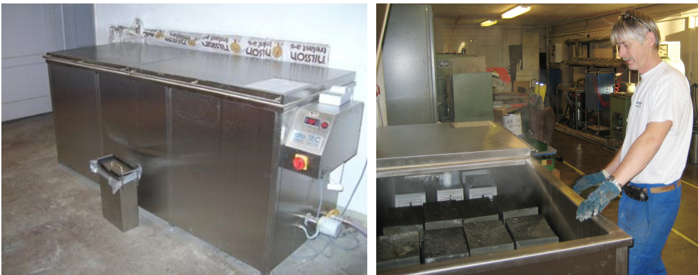
Photo 3-4—3-5 RILEM AAR-4.1: "Reactor" and storage container (see details in paper IV, Table 3). (Comment: Note the hot damp on the picture to the right when opening the lid of the "reactor". The stones to the right are used to press down the lid to get the new sealing completely tight – see photo 3-8).
