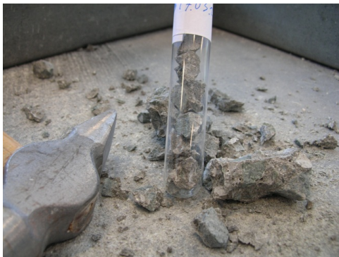
Photo 3-15—3-16 RF measurements; crushing of concrete (left) and glass tubes with Vaisala sensors (right).
