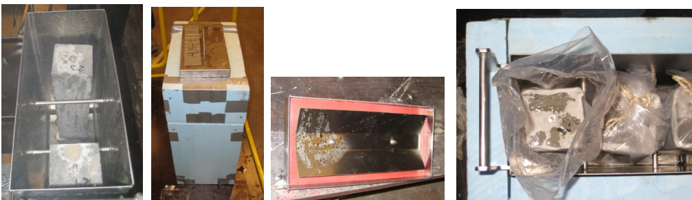
Photo 3-6—3-9 RILEM AAR-4.1: Storage container with unwrapped prisms (left), the insulated box used during measuring (middle left), the new sealing system (middle right) and wrapped prisms (right) (Comment: The water on top of the prism (right) is the 5 ml added before closing the polyethylene bag - see details in paper IV, Table 3.)
