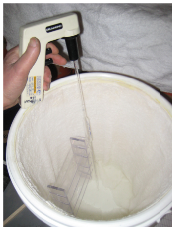
Figure 2-2. Sampling of water in a container by use of a pipette (left). Plastic bottle for storage of the water sample (right).
