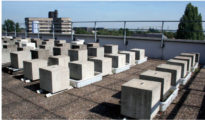
Fig. 3. Concrete cubes located at the outdoor exposure site in Düsseldorf, Germany.
