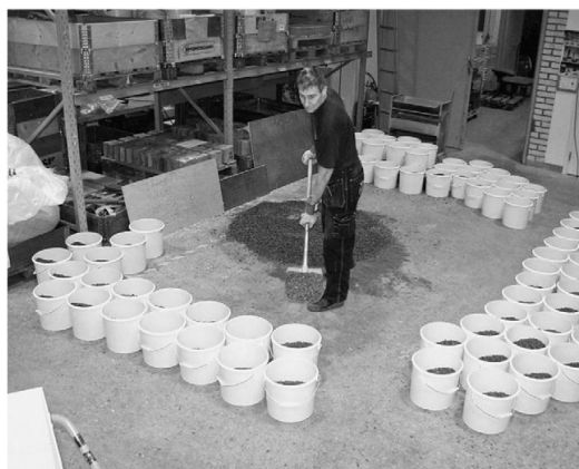
Fig. 19. Fractional shovelling, in accordance with EN 932-2.
