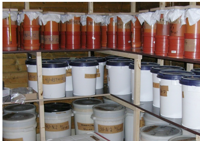
Photo 3-11 38°C storage room with containers for the RILEM AAR-3 CPT (top), the ASTM C1293 CPT (middle) and the Norwegian CPT (bottom).
