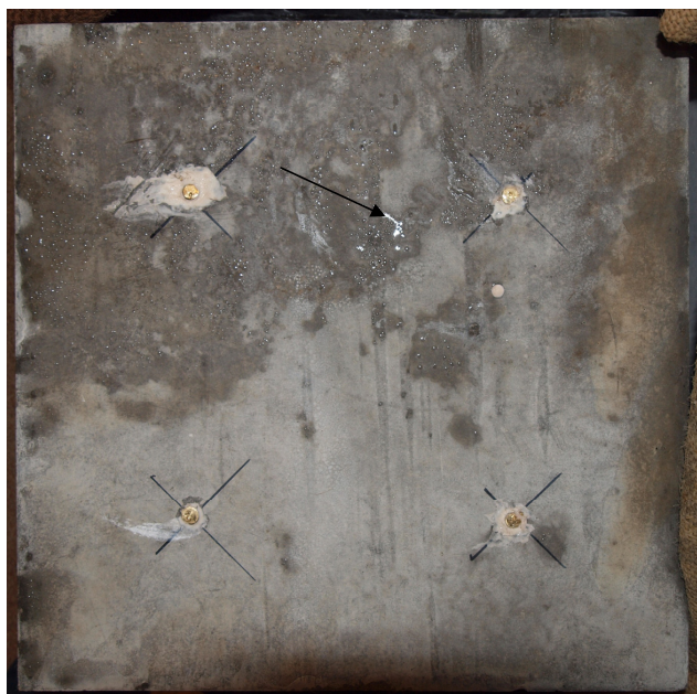
Figure 4. Top surface with brass screws glued in drilled holes. The arrow shows a measuring hole.
