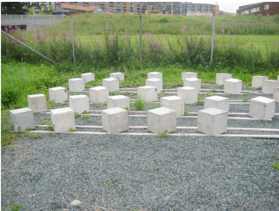
Photo 6-5 Field exposure site at SINTEF in Trondheim.
