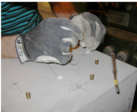
Photo 6-2—6-3 Preparation of measuring points (brass screws, glued in drilled holes; left) and final prepared cube including nameplate (right).
