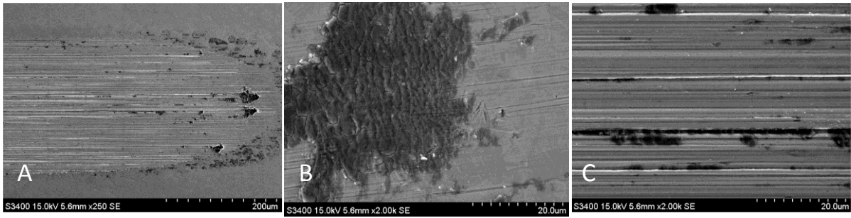
Figure 4-35: SEM images of wear track from CoCrMo PBS 7.4 tests. Magnifications: A x250, B x2k, C x2k
