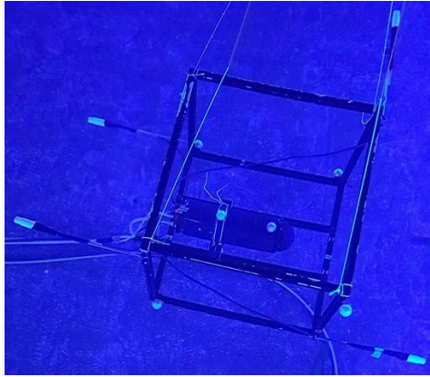
Figure 6.4: The sensor platform with hydroacoustic transducers (on rods), Qualisys markers (reflective balls), and an underwater housing. The blue light is emitted from the OQUS camera system in order to better detect the reflective markers.
