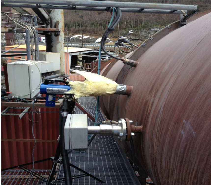
Fig. 4.10: The NEO LASERDUST and the FTIR is shown in this figure.
