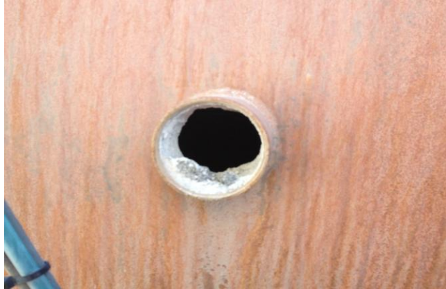
Fig..4.8: This figure shows the opening in the off-gas system where the FTIR was placed before the filter. The diameter needed for placing the FTIR in the off-gas system is 4cm. This opening is 9cm and is actually too big for the FTIR. Wool was used to cover the FTIR so that false air will not influence the results.
