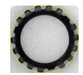
Fig. 2. View of a star washer from the top, highlighting the outer diameter.
