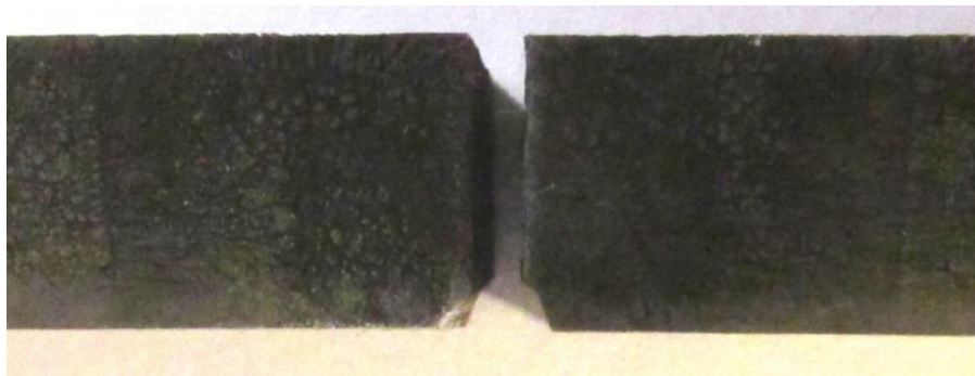
Figure 52: Macro photo of the HAZ of material A from test 2. Specimen fully separated by cracking.
