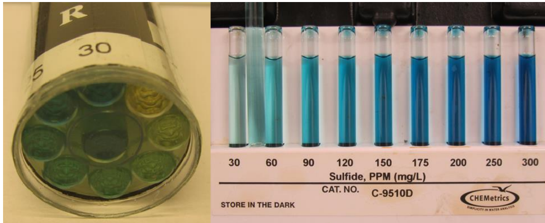
Figure 22: Sulfide content of electrolyte in test 1 at about 30 ppm, on a scale from 0 – 30 ppm and 30 – 300 ppm.
