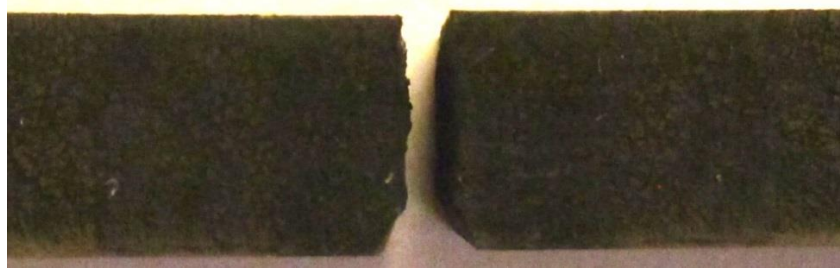
Figure 53: Macro photo of the HAZ of material B from test 2. Specimen fully separated by cracking.
