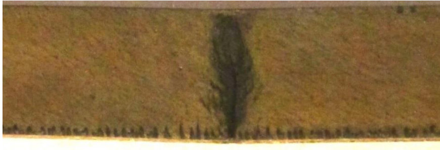
Figure 47: Macro photo of base material B, specimen from test 2. Severe cracking observed.
