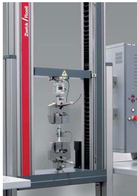
Figure 10: Zwick 30kN universal test machine, model Z030, used for tensile testing. [Zwick Roell]
