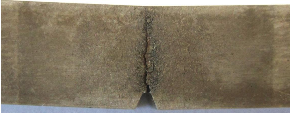
Figure 37: Macro photo of cracked specimen of simulated material B from test 1, crack lengths of 6.5 to 6.85 mm.
