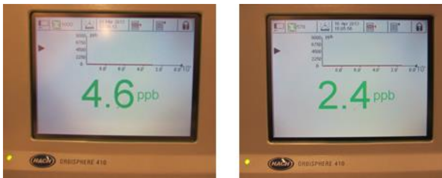
Figure 18: Documentation of oxygen level of 4.6 ppb in electrolyte for test 1 (left) and an oxygen level of 2.4 ppb in the electrolyte for test 2 (right). The O 2 -level was measured on the Obisphere 410 instrument.
