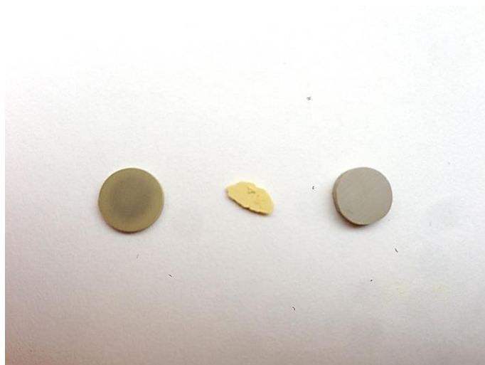
Figure 4.1.21 Photograph of annealed PSN pellets (Sample1-3). The samples were annealed for 42h at 1000°C (Sample1, left), 18h + 100h at 1100°C (Sample2, middle) and 18h at 1150°C (Sample3, right).
