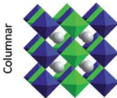
Figure 2.2.2 Columnar ordering of B-cations. Blue and green represents B'O_6 and B''O_6 octahedral sites [2].
