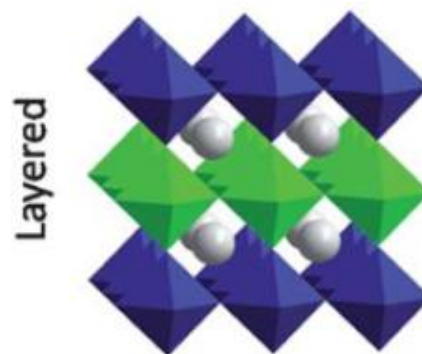
Figure 2.2.3 Layered ordering of B-cations. Blue and green represents B'O_6 and B''O_6 octahedral sites [2].
