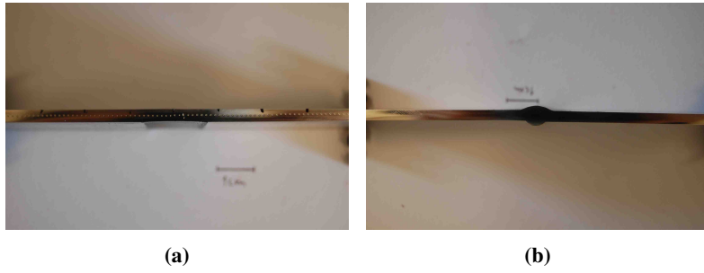
Figure 3.5: Photographs of weld samples used in the hardness testing: (a) FS welded sheets and (b) GMA welded sheets.
