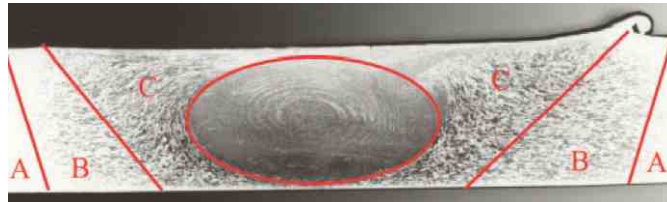
Figure 2.19: Microstructural zone classification in a friction stir weld [14].
