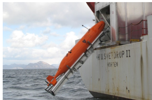
Figure 2.1: The HUGIN Autonomous Underwater Vehicle onboard H.U. Sverdrup II. Picture credited to Hegrenæs and Berglund (2009)
