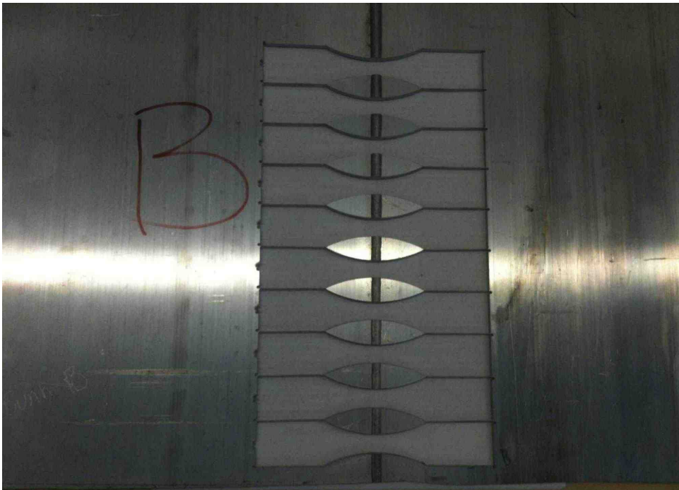
Figure B.4: How the specimens were taken out from one of the welded profiles. These specimens were post weld heat treated.
