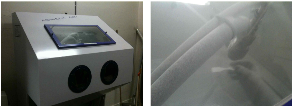
Figure 4.12: Shot peening of as welded specimens of AA6082.50-T6.
