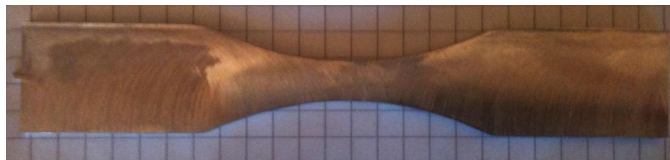
Figure 4.8: As welded specimen AA6082.50-T6.
