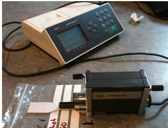
Figure 4.3: Mahr Perthometer M2 measuring the surface roughness of a shot peened specimen of AA6082.50.
