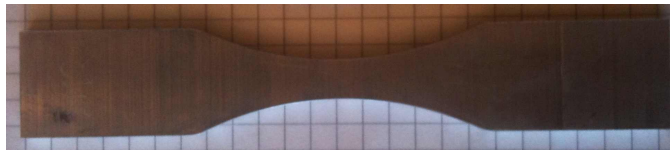
Figure 4.7: Base material specimen AA6082.50-T6.
