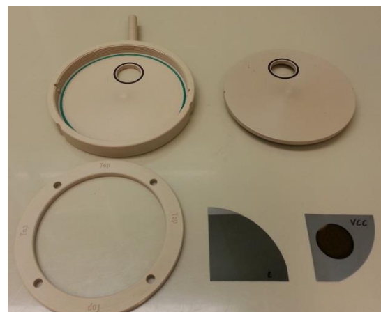
Figure 12: Disassembled sample holder for HF etching, including two quarter wafers, one non-etched (left) and one etched (right).
