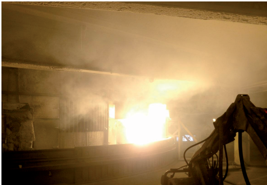
Figure 2-1: A picture of the tapping area at a silicon production plant shows that the capture of fume formed during tapping is not efficient. Photo: Mari Kirkebøen Næss.
