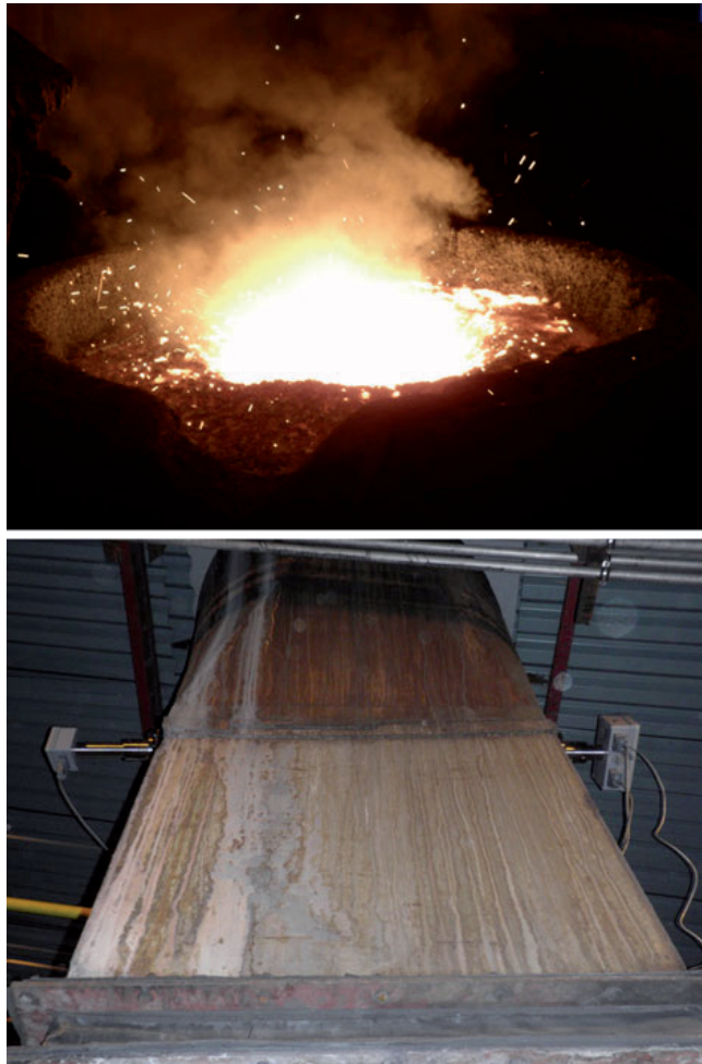
Fig. 3 Top: Photo of the top of a ladle with silicon being refined, showing the dynamic nature of the silicon surface and the air above. Bottom: Photo of the LaserDust MP installed at the off-gas channel
