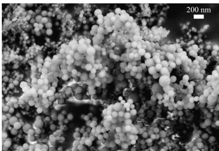
Fig. 9 SEM image of the fume deposits collected from inside the tube
