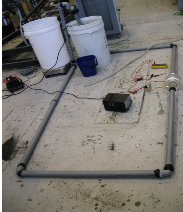
Figure.14 Photograph of experimental set-up constructed using DN 50 mm x 1.8 mm plastic pipe.
