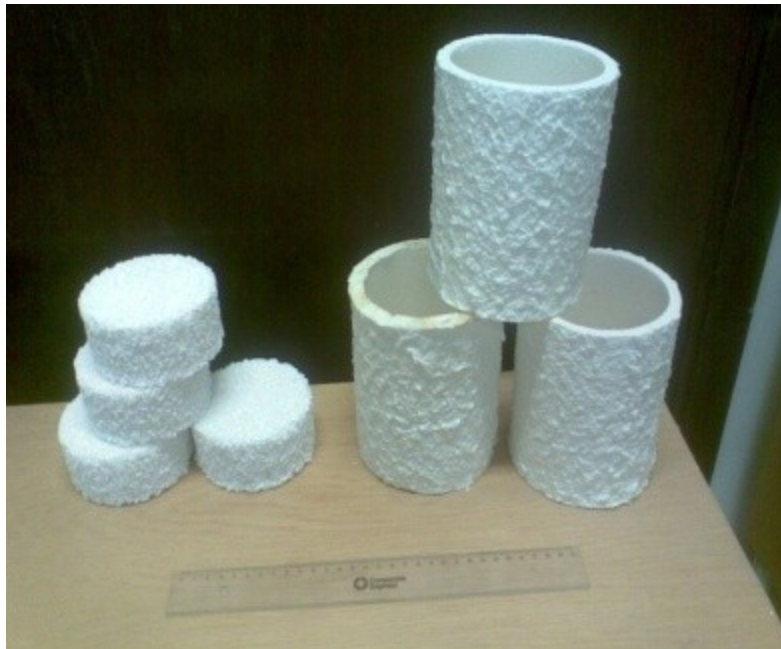
Figure.19 30 ppi Sivex ® CFFs (left side) and Bimex ® 400 insulated crucibles (right side).
