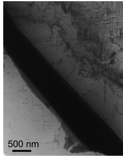
(b) A Ca-containing particle embedded in the Al matrix. Note the precipitate-free zone on the right side of the particle.
