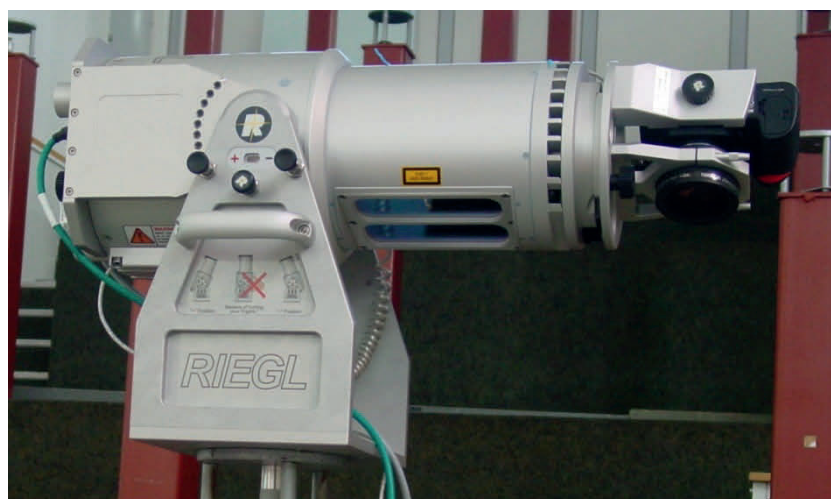
Figure 4.1: Picture of the laser scanner (Riegl LMS-Z420i) used in this work. Dimensions without camera: length 463 mm, diameter 210 mm, weight 16 kg.
