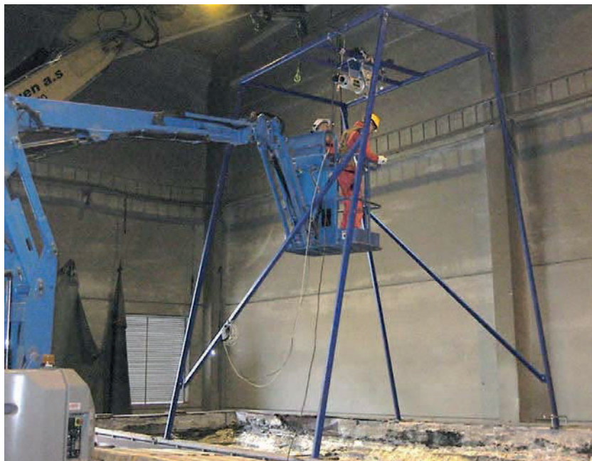
Figure 4.3: Mounting of the laser scanner on the rack, about 5 m above the cathode.
