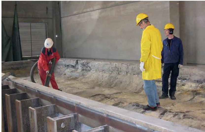
Figure 4.2: Prof. K.R. Holm and the author inspecting the cathode while Hydro employee, dr. J. Hajasova, vacuum-cleans the cathode before laser scanning.
