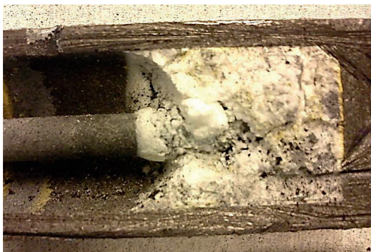
Figure 6.8: The bottom of the reference electrode during autopsy. A cross-sectional cut revealed that some parts were corroded away during the experiment. The alumina crucible which should have been at the bottom was gone, as was the aluminium inside it. Furthermore it was found that the tungsten current lead was corroded several cm up into the insulating alumina tube, which means that the electrical contact probably has been broken at some point during the experiment.
