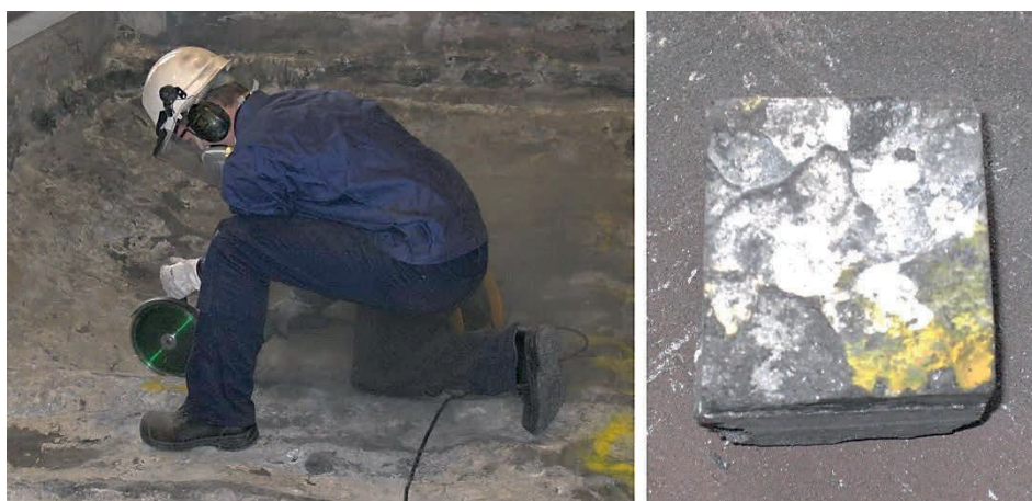
Figure 5.1: The author extracting samples from the cathode with an angle grinder. The sides of the cuboid samples were typically 3–5 cm.
