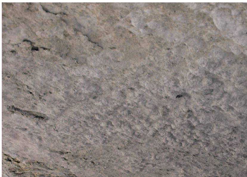
Figure 2.33: Solidified metal pad removed from a terminated cell at Qatalum. The picture was taken from beneath the metal pad, held up by a crane. The metal and bath remnants act as a cast of the cathode surface, showing the inverted pattern. The bumps in the lower right area on the photograph correspond to the holes or dimples in the cathode surface. Yellow flakes and dust, i.e. aluminium carbide, can also be seen. Photo: S. Jarek, Hydro.
