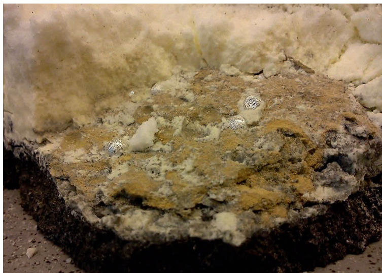
Figure 6.13: A picture of aluminium carbide and metal droplets at the bottom of the crucible.
