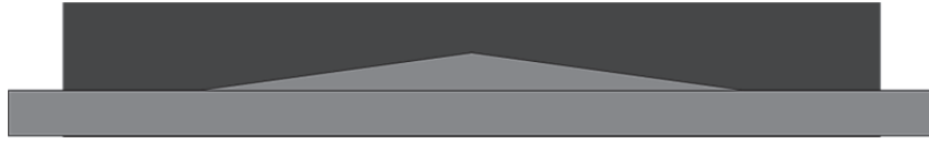
Figure 7.8: Sketch of a cathode block and a current collector bar with triangular profile.
