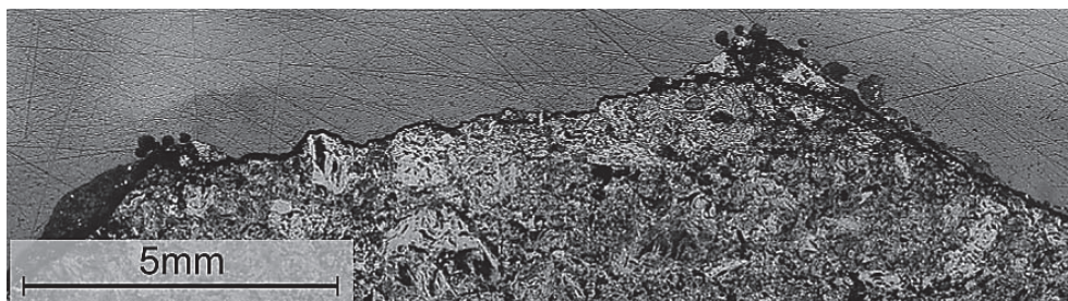
Figure 5.24: An overview picture of the surface of a sample from a GZ cathode block, put together by several optical micrographs. The rough surface is probably a result of particle detachment due to carbide formation and wear in the superficial porosity.
