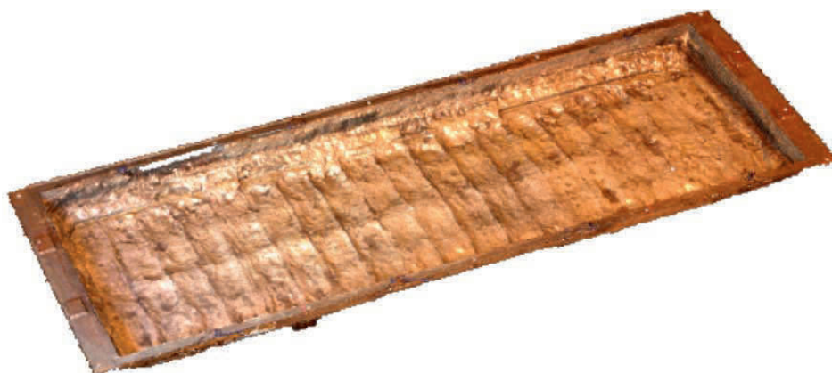
Figure 4.4: A 3D model of cell D105, where the coordinate data points have been ascribed RGB colour values from the photographs taken by the camera mounted on the laser scanner.
