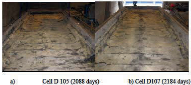
Figure 1. Cathode surfaces of cell D105 (a) and Cell D107 (b).
