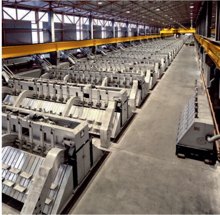
Figure 1.1: Image from pot room SU4 at Hydro Sunndal, Norway, showing a side-by-side line of aluminium reduction cells coupled in series. The current pass through the anodes at the top of the cell to the cathode at the bottom, and then up to the anodes of the next cell in the line. One pot line may consist of more than hundred cells (or pots). Photo: A. Johansen. © Norsk Hydro
