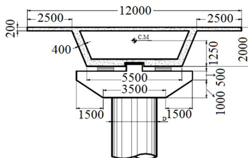
Figure 1– Cross section of the bridge [5].
