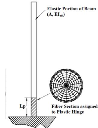
Figure 2 – Fibre hinge [9]
