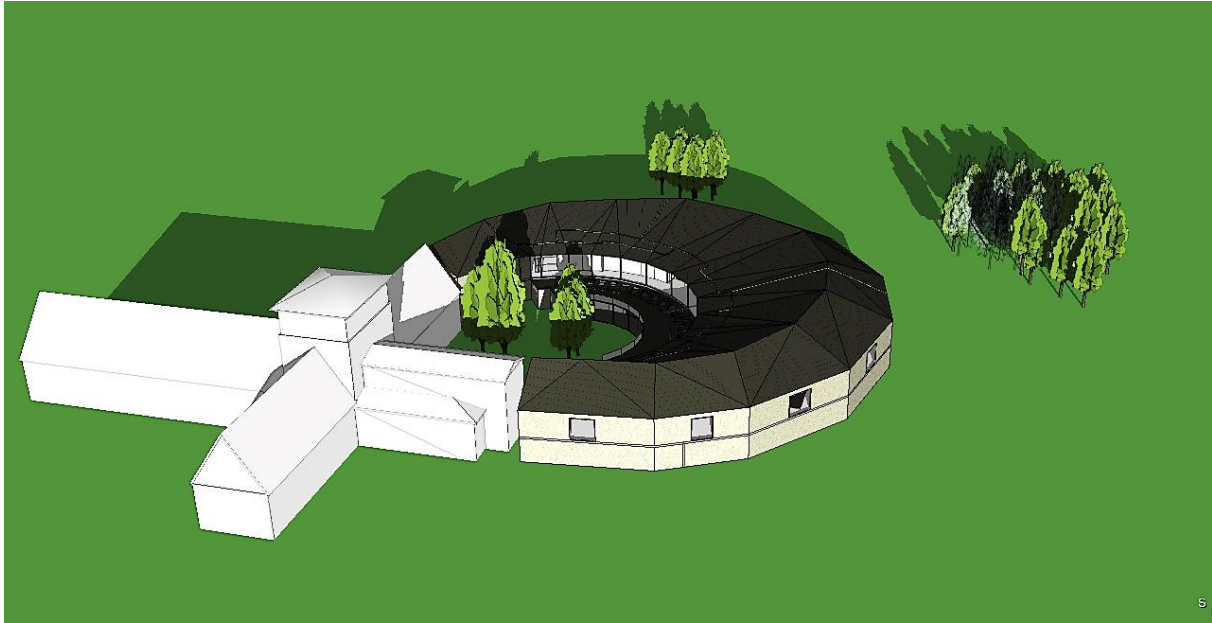
Figure 26: 3D model in IDA ICE with shading from trees and old museum building
