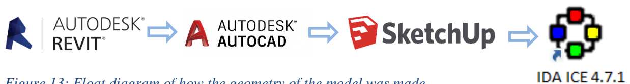
Figure 13: Float diagram of how the geometry of the model was made
