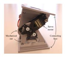
Fig. 1. 3D printed GZ-I module.
