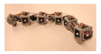
Fig. 7. Screw-less assembly of a snake-like robot.
