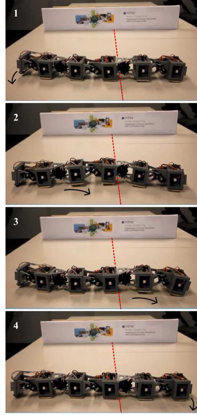
Fig. 10. Snapshots of onsite sidwinding locomotion experiment in one period. The red line is used as a reference for observing displacement.
