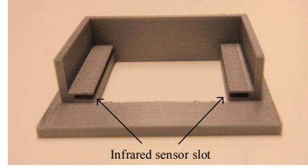
Fig. 5. Terminal module for head/tail infrared sensor mounting.
