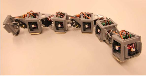
Fig. 7. Screw-less assembly of a snake-like robot.
