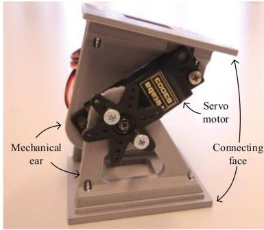
Fig. 1. 3D printed GZ-I module.
