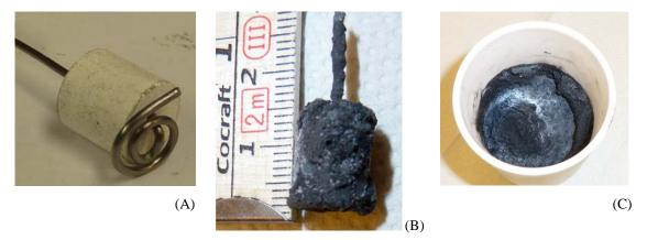
Figure 3. Examples of the Sc<sub>2</sub>O<sub>3</sub> pellet (cathode) (A) before and after (B) electrolysis. C) alumina crucible and frozen electrolyte with carbon layer on top after electrolysis.
