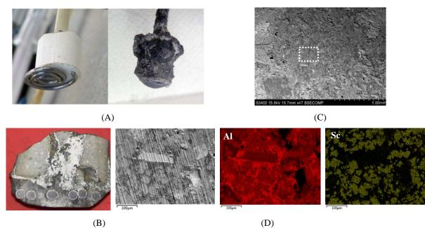
Figure 4. A) Picture showing the  $Sc_2O_3$  precursor in contact with  $Al_2O_3$  before and after the electrolysis; B) Cross section of the  $Sc_2O_3$  precursor after electrolysis, showing the formed metal phase; C) Back scattered electron image of the metallic part, and D) EDS analysis of the zoomed image.
