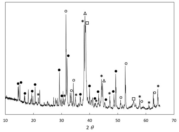
Figure 5. XRD diffractogram of the metal product showing the formation of ScAl<sub>3</sub> intermetallic compound. (\*) Al3Sc; (O) Sc2O3; ( $\bullet$ ) CaCl2 (H2O)2; ( $\triangle$ ) Al; ( $\Box$ ) Ta. It is important to notice that the cathode product was not washed prior to the analysis, so remains of electrolyte are still present.
