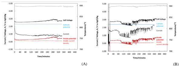
Figure 2. Electrolysis parameters recorded during the reduction of Sc<sub>2</sub>O<sub>3</sub> precursors when applying: A) -2.3 V; and B) -2.4 V versus AgCl/Ag reference electrode system.
