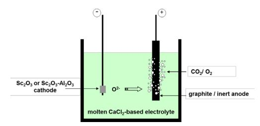
Figure 1. Schematics of the FFC process applied to Sc and Sc-Al reduction directly from their oxides.
