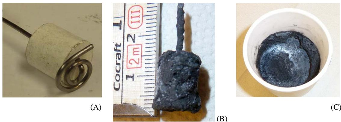
Figure 3. Examples of the  $Sc_2O_3$  pellet (cathode) (A) before and after (B) electrolysis. C) alumina crucible and frozen electrolyte with carbon layer on top after electrolysis.
