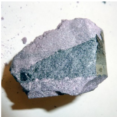
Figure 4 Picture of the salt after one of the electrolysis experiment
