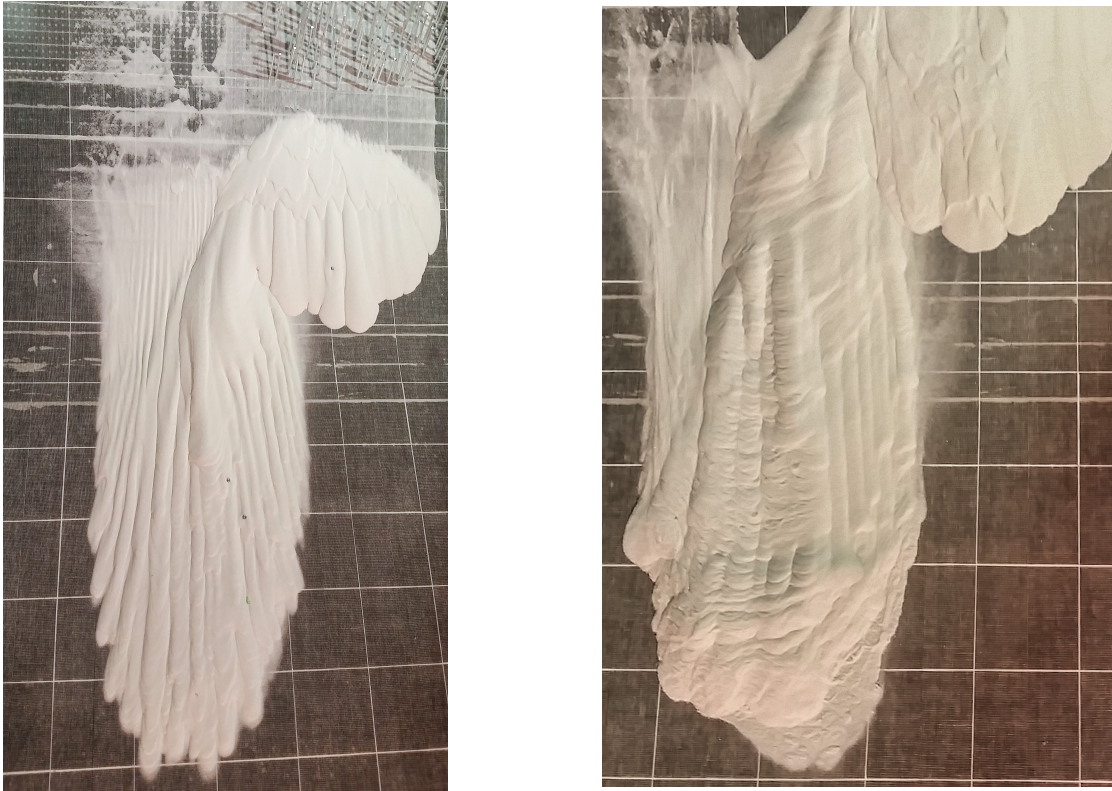
Figure 5.7: Ballotini at 50% (left) and 70% relative humidity (right).
