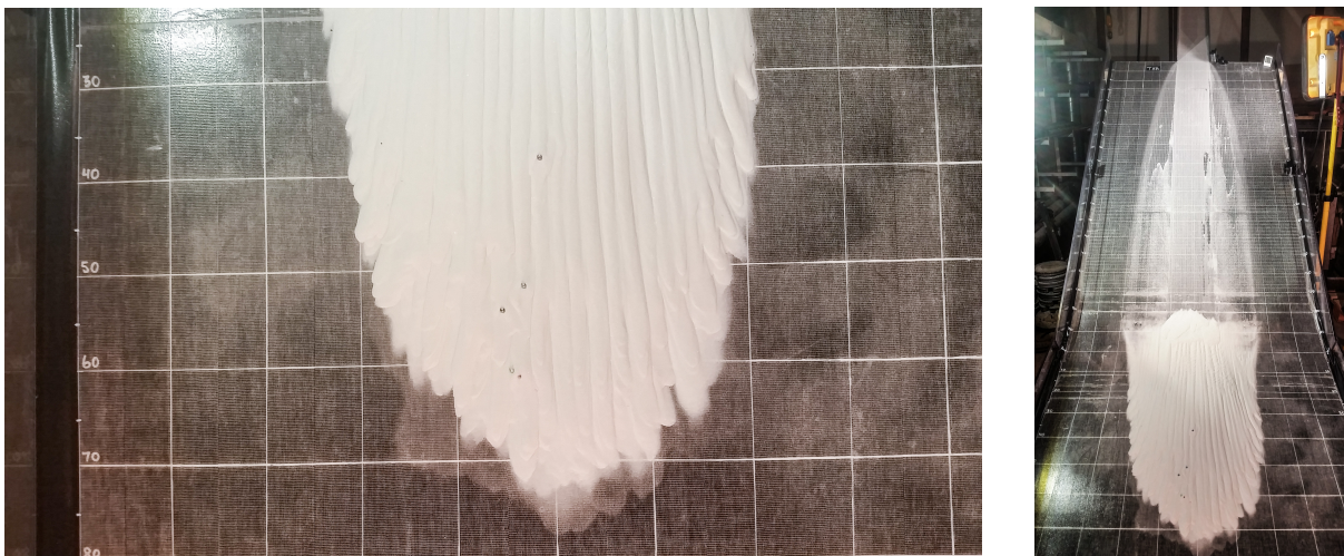
Figure 4.7: Ballotini reference trials showing blown-up runout distance alongside the chute view.
