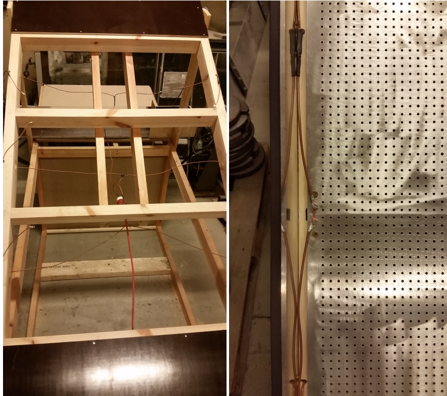
Figure 4.2: Static discharge from 12 points of contact to the grounding rod.
