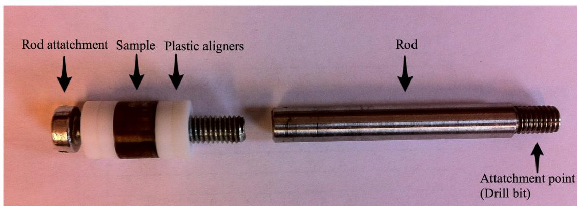
**Figure 3.3:** Sample holder for pre treatment of cylindrical steel samples used in polarization experiments. All metallic parts made in carbon steel to avoid galvanic couplings.
