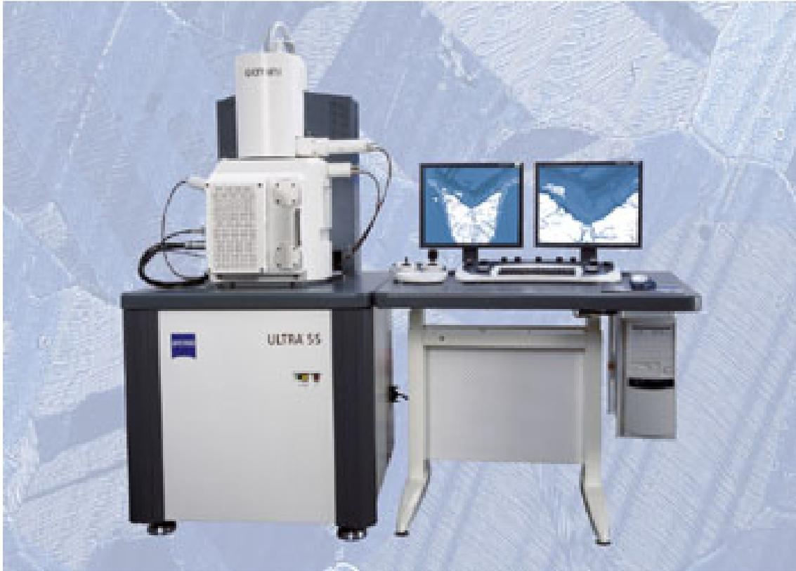
**Figure 3.11:** Zeiss Ultra 55 limited edition (FESEM). Field emission scanning electron microscope used for surface characterizations throughout experiments.
