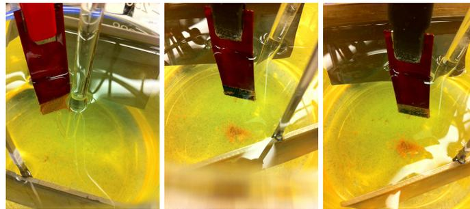
(e)  $i_{AC} = 100A/m^2$ . 24h into experiment. (f)  $i_{AC} = 100A/m^2$ . 6 days into experiment. (g)  $i_{AC} = 100A/m^2$ . 7 days into experiment.
