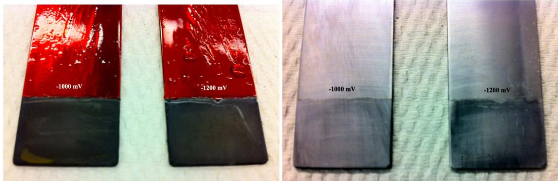
(c) Samples before post-treatment ( $i_{AC} = 500 A/m^2$ ) (d) Samples after post-treatment ( $i_{AC} = 500 A/m^2$ )
