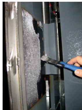
Figure 10. Mechanical removal of wax deposit layer from a cold bare steel test-section.
