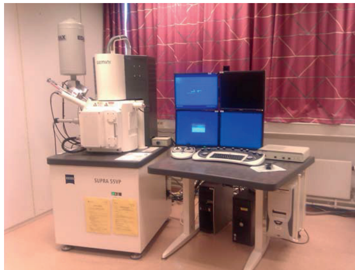
Fig. 3. Photograph showing the Zeiss Supra 55 VP SEM.
