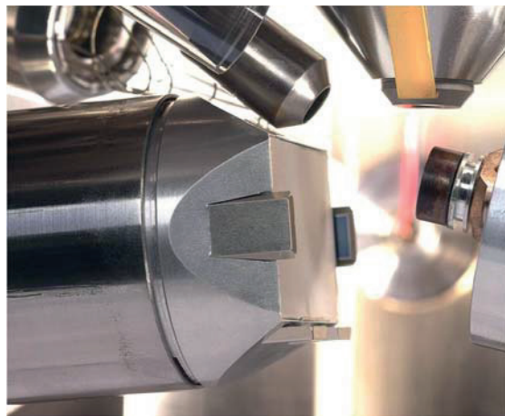
Fig. 14. Micrograph of typical EBSD hardware inside the SEM chamber ( www.ebsd.com ).
