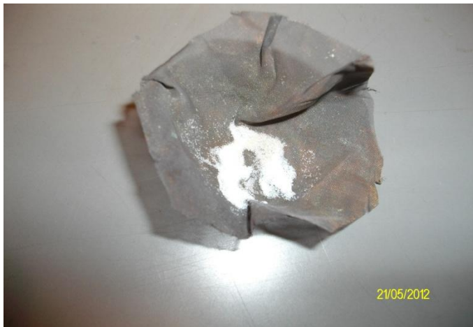
Figure 17 Frustules on stainless steel grid
