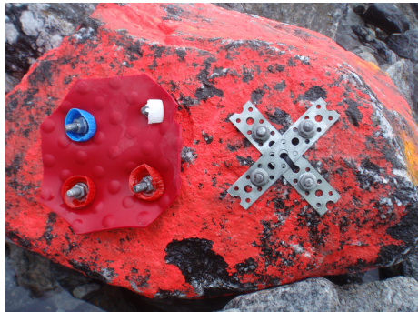
(c) Smartstone probe mounted in a stone used for the model tests (Photo: NTNU) (d) Riprap stone equipped with a Smartstone probe (left) and a pressure cell (right) (Photo: NTNU)
