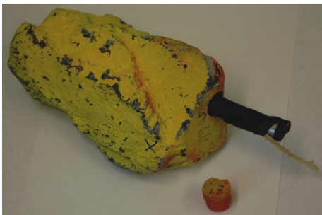
(c) Smartstone probe mounted in a stone used for the model tests (Photo: NTNU) (d) Riprap stone equipped with a Smartstone probe (left) and a pressure cell (right) (Photo: NTNU)
