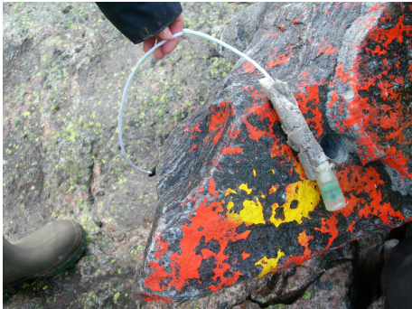
(a) Accelerometer removed from a riprap stone after the field experiment F13P2 (Photo: NTNU) (b) Smartstone probe with size indication (Photo: O. Gronz)
