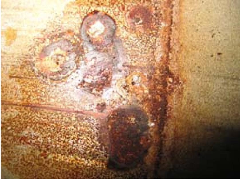
**Figure 3.3: Picture of crevice corrosion found under a tag from an offshore installation in the North Sea.**
