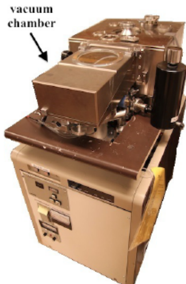
Fig. 1. The external vacuum chamber used to design and test the potential of gas quenching.
