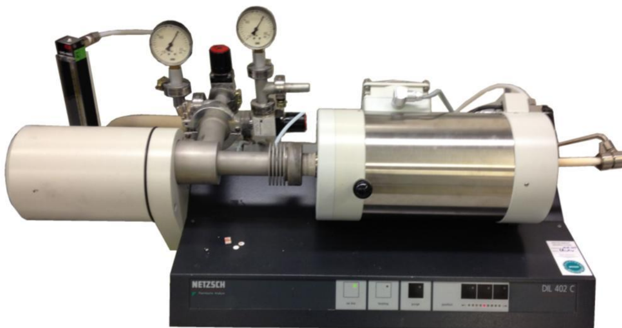
Figur 19: Figuren viser Netzsch DIL 402 C dilatometer.
