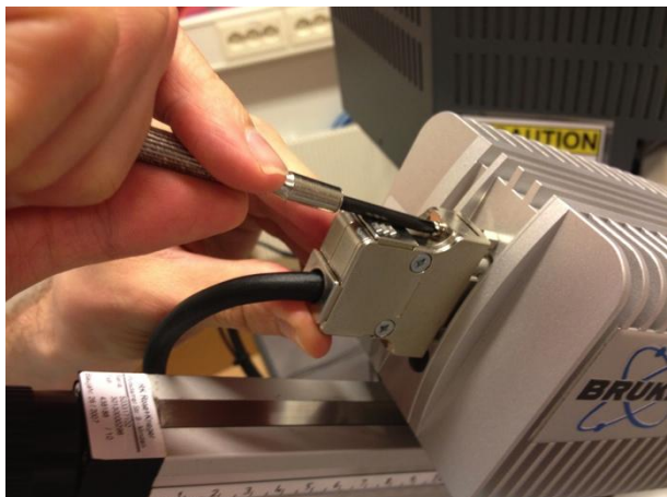
Figure 11: Removal of the EDS signal cable.
