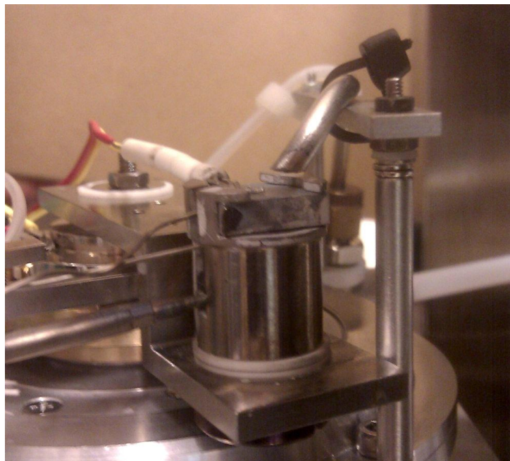
Figure 18: After the quenching rig has been installed inside the SEM the in situ hot stage may be mounted to the SEM stage. The stainless steel tube is adjusted and the distance between the gas outlet and the sample is minimized.
