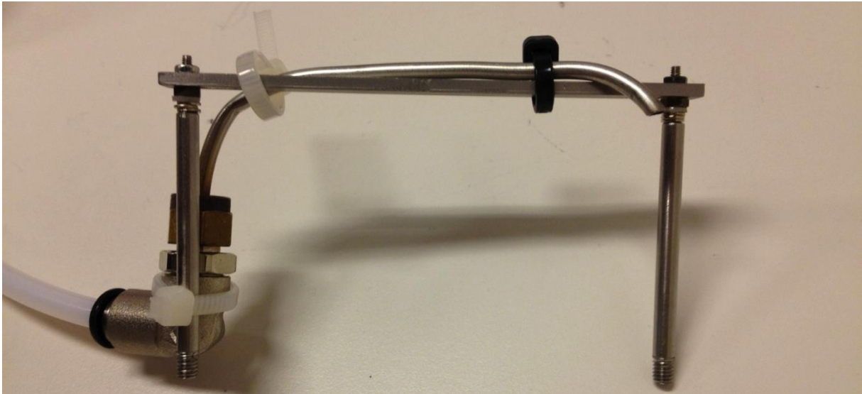
Figure 8: The stainless steel quenching tube fitted onto the quenching rig.
