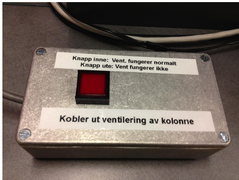
Figure 7: Ventilation switch for disabling of the normal SEM ventilation system.
