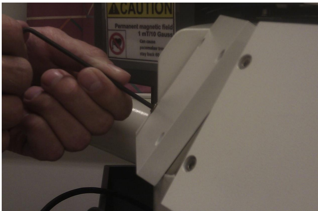
Figure 13: Replacing the EDS-detector with the SEM port cover.
