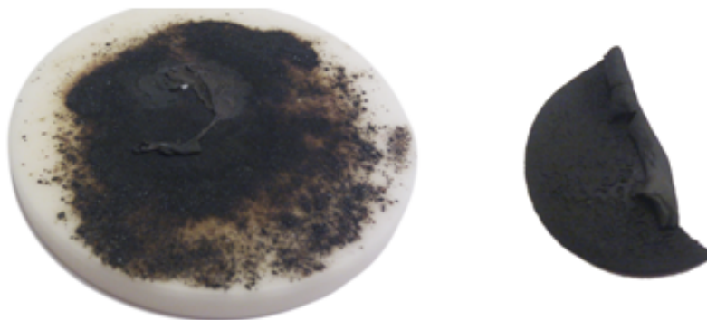
Figure 4-13: Remains of two broken and disfigured LSFTa_32CB-substrates
