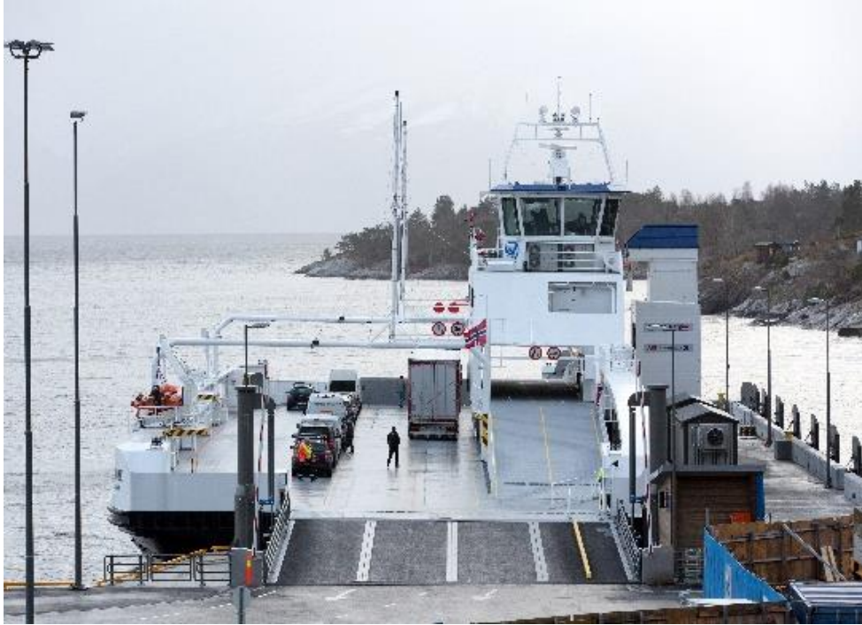
Figure 8: MS Ampere at port charging (Stensvold, 2015).
