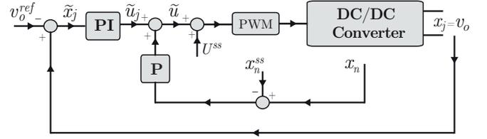
Figure 1. Control block diagram.
