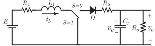
Figure 2. Circuit diagram of the boost converter.
