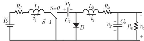
Figure 4. Circuit diagram of the cuk converter.
