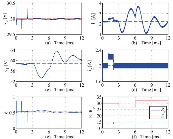
Figure 5. Simulation results for the cuk converter: (a) output voltage, (b) first inductor current, (c) first capacitor voltage, (d) second inductor current, (e) duty cycle, and (f) source voltage and load resistor.
