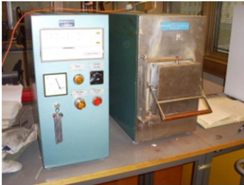
Figure 10-- Muffle furnace used for oxidation experiments.
