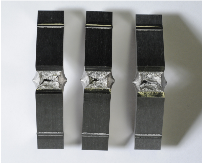
Figure 36: Charpy specimens 1-3 from the right. Heat treated at 1120^{\circ}\text{C} . Specimens showed an average Charpy toughness value of 297 J and ductile fractures with rough fracture surfaces and lateral expansion on both sides of the specimens.
