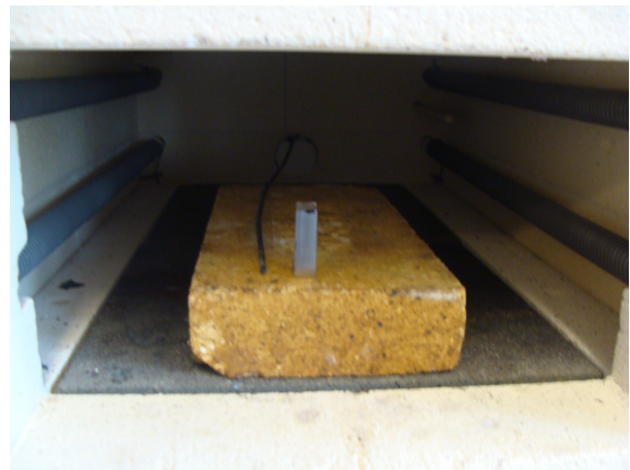
(b) Specimen and thermometer positions in the furnace
