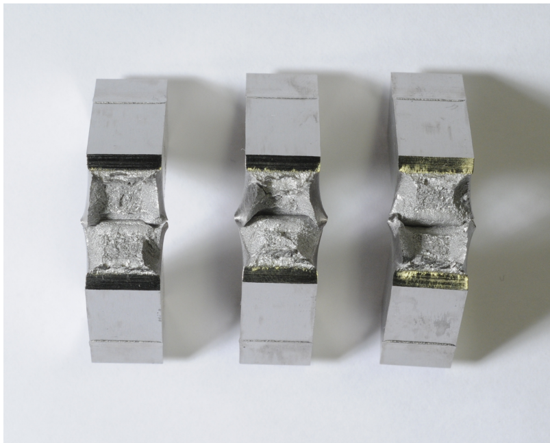
Figure 37: Charpy specimens 4-6 from the right with Charpy values of 192, 280 and 170 J respectively. Heat treated at 1160^{\circ}\text{C} . Specimens showed an average Charpy toughness value of 214 J and less ductile fractures than the other specimens.
