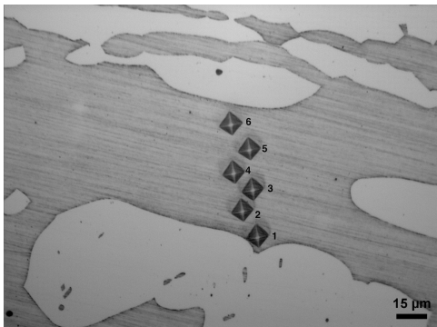
(c) Hardness indentations across ferrite band of 69 \mu\text{m} . Sample C heat treated at 1120 ^{\circ}\text{C} .
