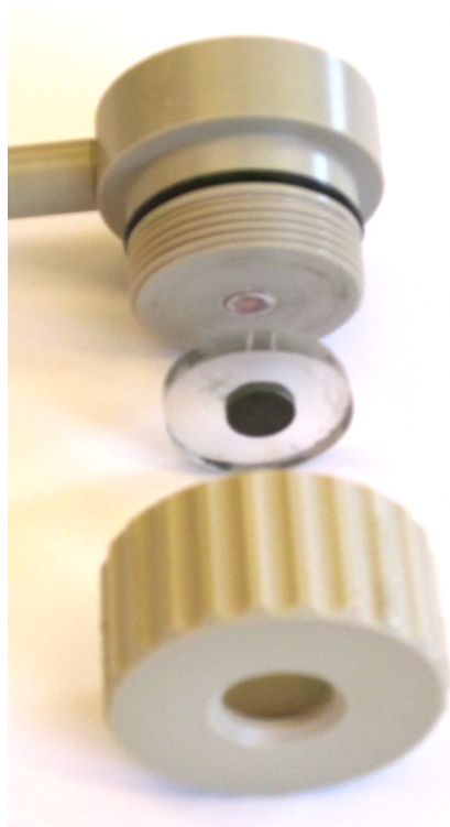
Figure 9: This figure shows how the pellet samples are mounted to the sample holder. Colloidal solved silver is added between the copper contact and the pellets backside in order to ensure good electronic contact.
