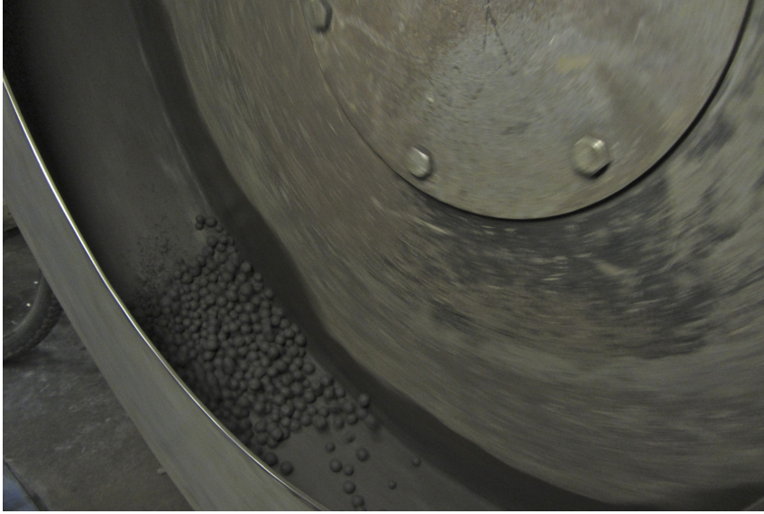
Figure 4.1: Laboratory size pelletization drum.
