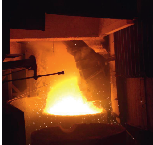
Figure 6.11: Tapping with "DogHouse" installed
