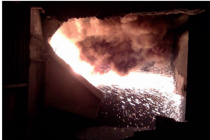
Figure 6.14: Fumes during initial oxygen lancing
