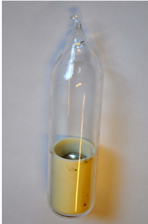
Figure 3.2: Vacuum capsule with alumina crucible inside.
