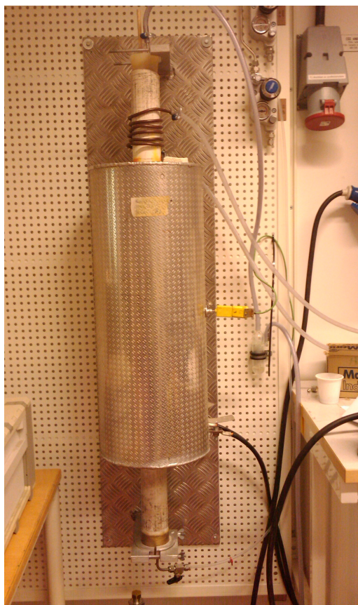
Figure 3.3: Vertical resistance furnace used for production of amorphous and crystalline BMG.
