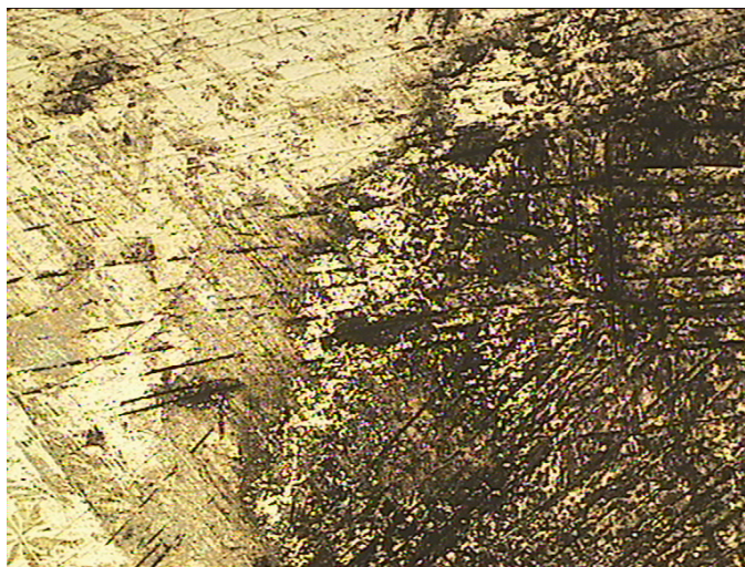
Figure 6.71: Corrosion on the surface of the crystalline zirconium based bulk metallic glass in PBS solution. T=37°C; pH=7.4; Magnification 50X.
