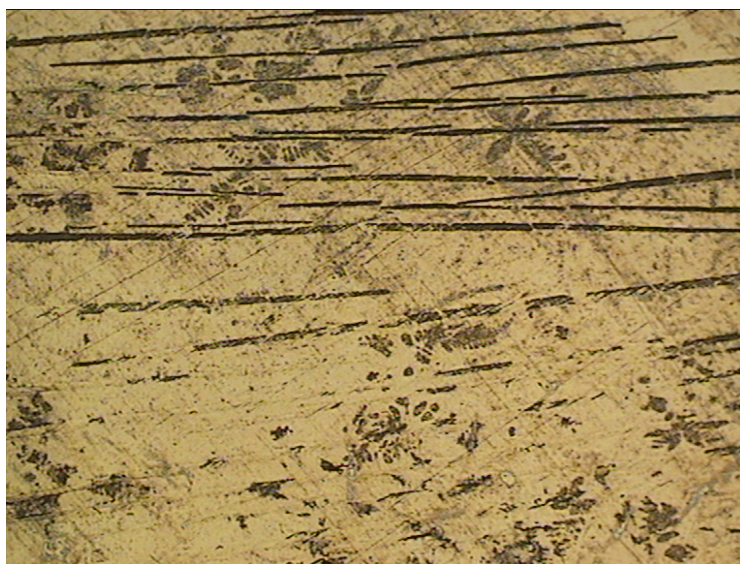
Figure 6.69: Corrosion on the surface of the crystalline zirconium based bulk metallic glass in PBS solution. T=37^\circ\text{C} ; \text{pH}=7.4 ; Magnification 100X.
