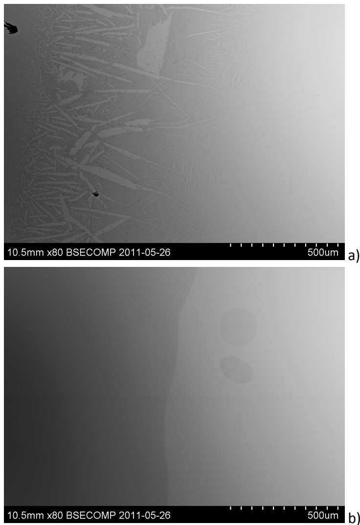
Figure 4.1: SEM image of the bulk metallic glass. (a) near the edge (b) the center of the sample.
