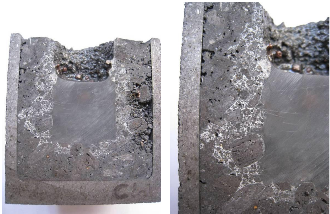
Figure 4.8: Crucible after experiment C.1d). Left: Intersected crucible. Right: Close-up of left half.
