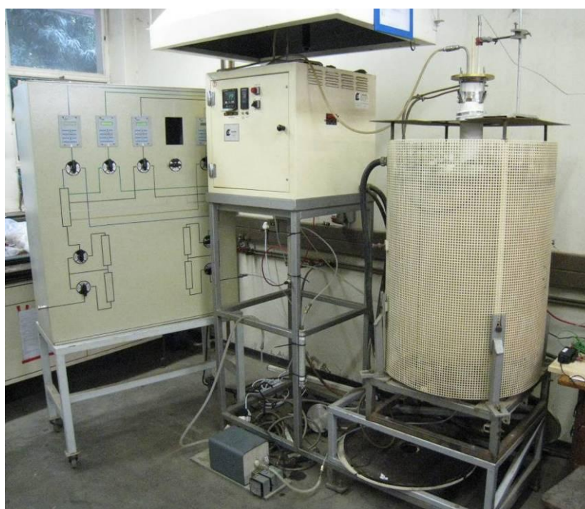
Figure 3.1: Furnace setup including (from left) mass flow controller, furnace controller and Carbolite tube furnace. On the floor: Zirconium gas purifier.
