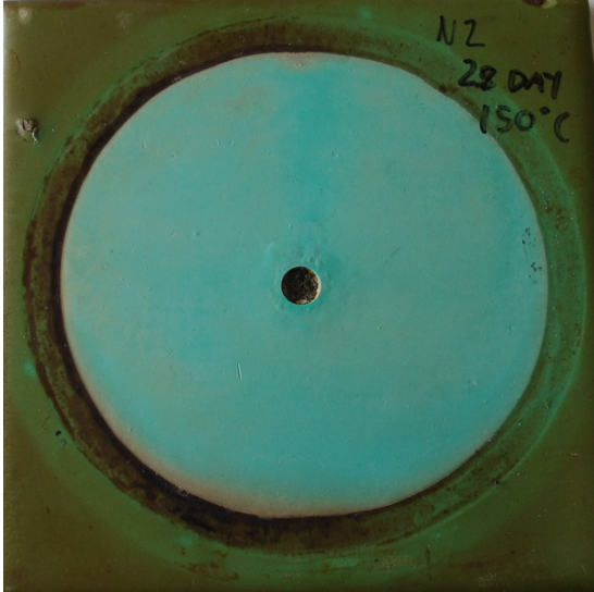
(a) Product N, blistering in the disbonded area
