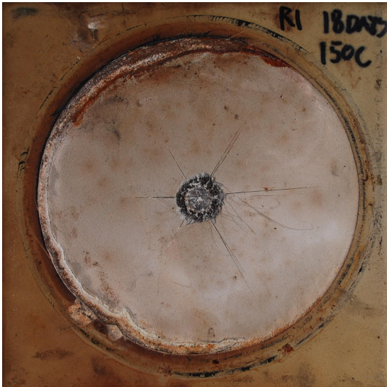
(c) Product R, Showing damage along the edge
