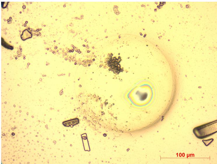
(b) The silicon have covered the entire frustule. Iridescence is visible on top of the silicon structure, and debris is laying around on the substrate beneath the silicon.
