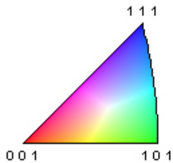
Figure 4.39: IPF translating the colours of a IPF map in to crystallographic orientations.
