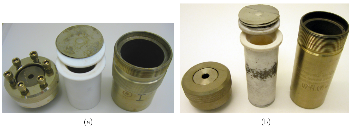
Figure 3.1: Pictures of 125 ml (a) (adapted from Sortland [1]) and 45 ml (b) autoclaves. For reference, the steel container widths are 8 cm (a) and 5 cm (b), respectively.
