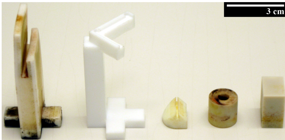
Figure 3.2: Pictures of substrate holders including from left to right: Large vertical, large horizontal and small vertical substrate holders, cylindrical and prismatic supports.
