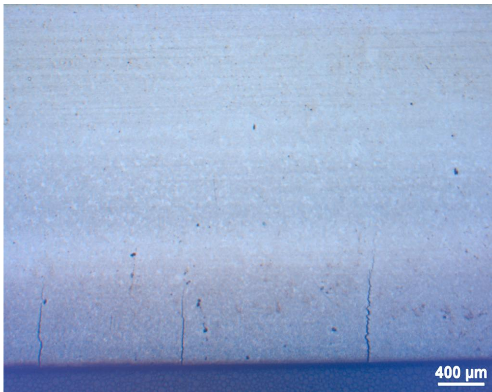
Figure 22. Low magnification image of a sample that was carburized at carbon potential of 1.3%. The dark blue layer at the bottom of the picture is the Clarocit cast material. Three cracks can be seen from the surface of the sample and stretching in towards the sample core.
