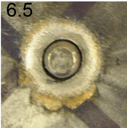
Figure R. Projectile entry and exit holes for shot 4 and entry hole for shot 5 on sample 6. Exit hole for shot 5 was not photographed.
