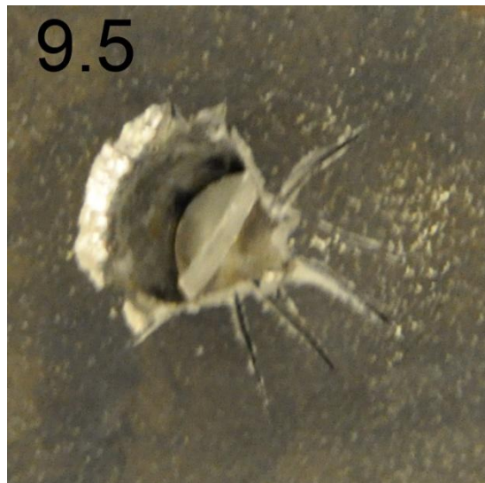
Figure X. Projectile entry and exit holes for shots 4 and 5 on sample 9.
