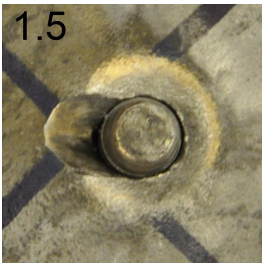
Figure H. Projectile entry and exit holes for shots 3, 4 and 5 on sample 1.
