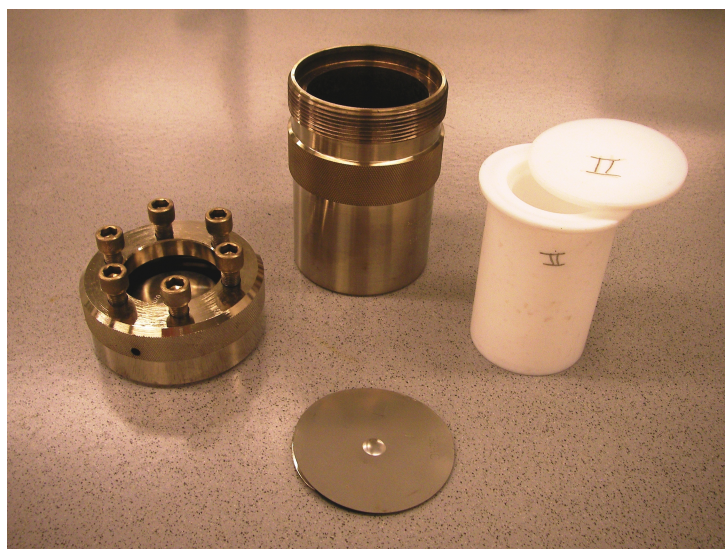
Figure 3.2: Image of the autoclave Parr 4748 Large Capacity Bomb and its components.
